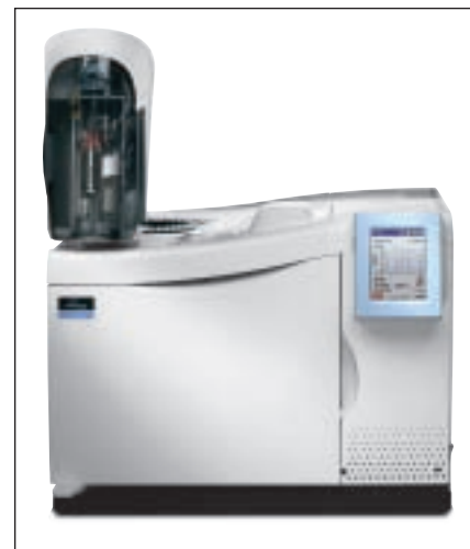
Figure 3. Clarus Gas Chromatograph.
