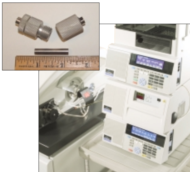
PerkinElmer HPLC/ICP-MS system. A small column developed for fast HPLC separations is shown.
