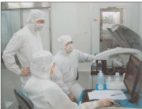
Our semiconductor team measures high purity samples using an ELAN DRC II in our class 100 clean room.
