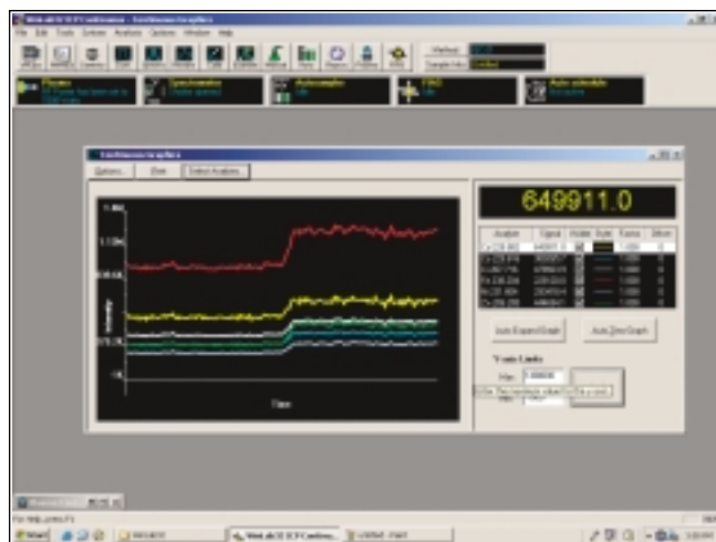
The Optima 2100 DV is capable of acquiring and displaying data in a continuous real-time graphics format. This is quite useful for optimizing instrument performance. The graph shows the signal increasing as the RF power is increased while data are being displayed.
