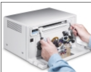
Figure 6. Easy interchange of FIMS absorption cell.
