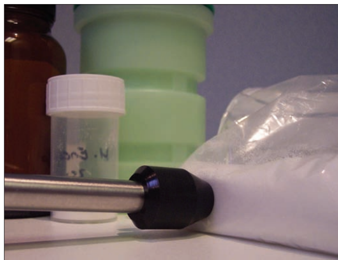
Figure 2. The nosepiece eliminates stray light and keeps the sample at the optimum focal distance from the probe.
