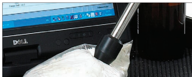
Figure 2. The nosepiece eliminates stray light and keeps the sample at the optimum focus distance from the probe.
