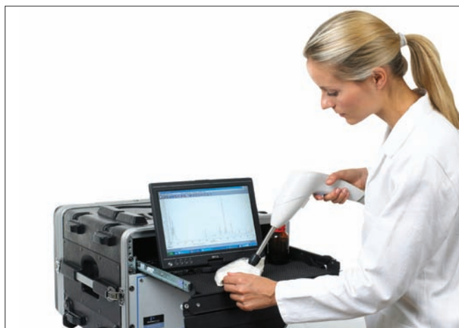
Figure 1. A triggered probe makes it easy to analyze a wide range of sample types at the scene or in a laboratory.
