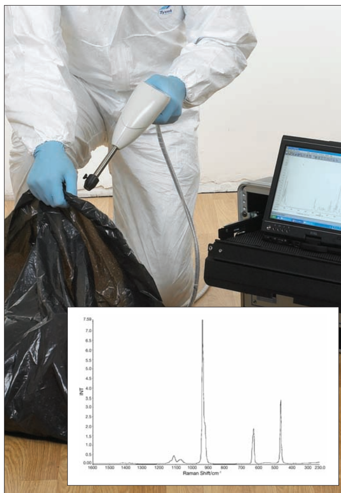
Figure 6. Raman spectra can be obtained through a variety of containers including black plastic bags. The spectrum is of ammonium perchlorate explosive through black plastic bag.
