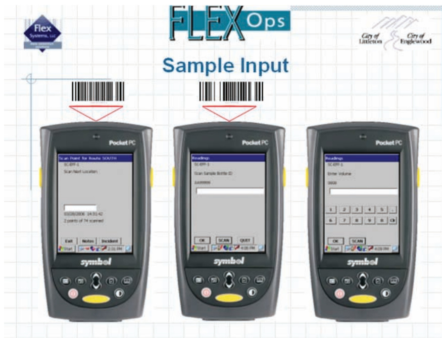
Figure 2. The FlexOps PDA application provides sample collection operators an easy-to-use data entry interface that automatically uploads collection information to LABWORKS.
